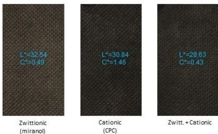
Fig. 1.1: Cold padding in acidic surfactant + electrolyte.
