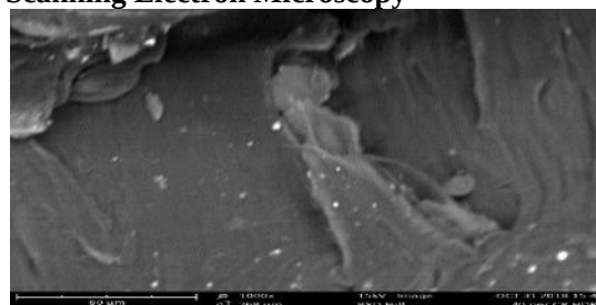
Fig. 5: SEM image of CP/HDPE composite A at 40% filler loading with coupling agent
