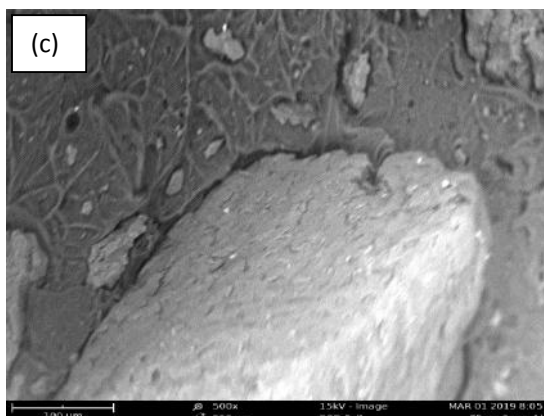
Figure 10: SEM micrograph of fracture surface of tensile strength specimen at 750 \mu\text{m}
