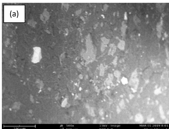
Figure 8: SEM micrograph of fracture surface of tensile strength specimen at 63 \mu\text{m}
