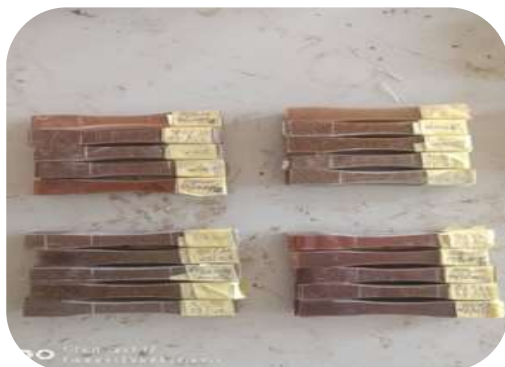
Plate 1: Fabricated Composite Sheets and Cut Tensile Samples for Analyses
