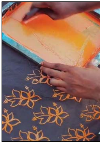
Step 5: place mesh on fabric and print
