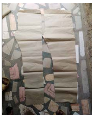
Plate 5: Front and back pattern of male trouser
