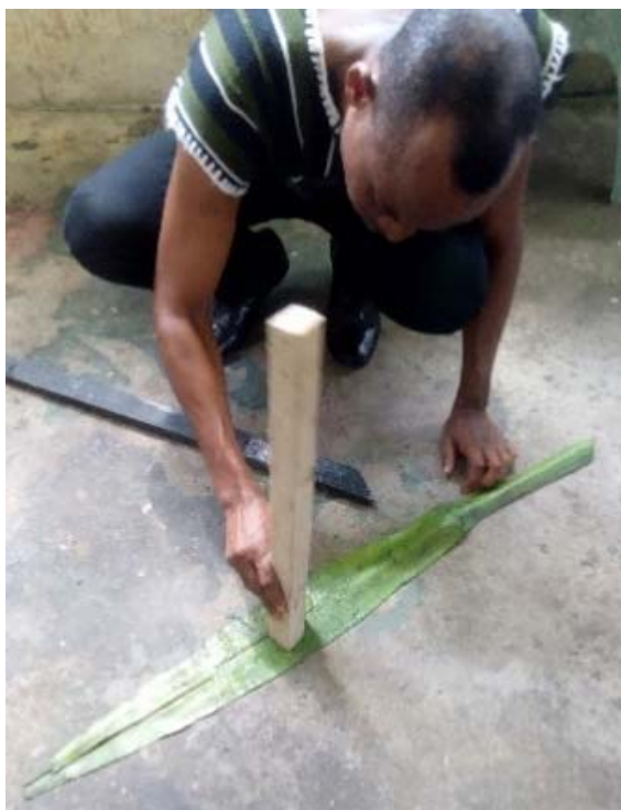
Fig. 2: Beating the heated sisal leaf to soften Source: Umana Nnochiri (2023)
