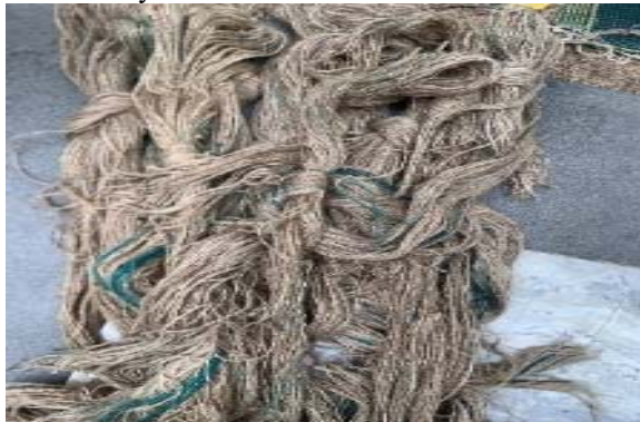
Fig 5. Unravelled Jute strands after fibre extraction, Medium: photography, Source: Ayuba Rejoice Betimaniu 2024
