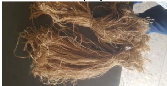
Fig 6. Uniform and aligned Jute strands after carding, Medium: photography, Source: Ayuba Rejoice Betimaniu 2024
